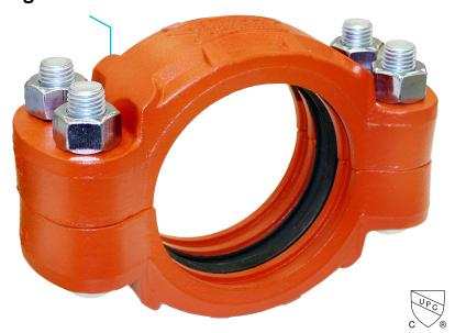
Gruvlok Fig. 7377 is a flexible coupling utilizing double groove technology designed for high pressure piping applications. Fig. 7377 is specifically designed for use in mining, oil, gas, slurry, sludge, and hydraulic systems. The maximum working pressure for each pipe schedule and size are listed in the table below. Fig. 7377 is an ideal solution for high pressure applications, exceeding ASC's Fig. 7004 capabilities. See page 3 for double groove piping dimensions.
